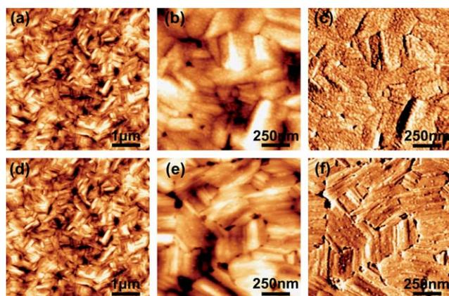
**Fig. 8** AM-AFM images (ambient conditions,  $512 \times 512$  pixels) of FG1:[70]PCBM (1 : 1.5), with different post-deposition annealing temperatures. (a, b, c) 5 mn at  $90^\circ\text{C}$ . (a) Topography,  $5 \mu\text{m} \times 5 \mu\text{m}$ . (b, c) topography and phase,  $1.25 \mu\text{m} \times 1.25 \mu\text{m}$ . (d, e, f) 5 mn at  $120^\circ\text{C}$ . (d) Topography,  $5 \mu\text{m} \times 5 \mu\text{m}$ . (e, f) Topography and phase,  $1.25 \mu\text{m} \times 1.25 \mu\text{m}$ .
