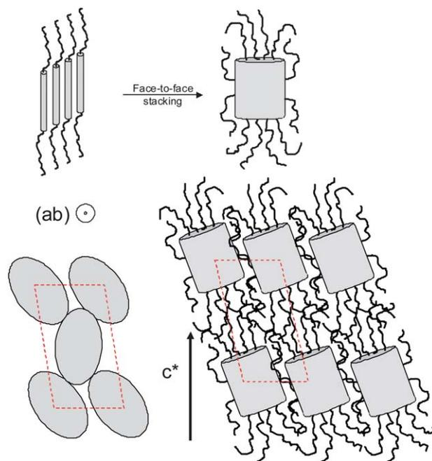
**Fig. 5** Proposed model of the 3D smectic phase ( $\text{Sm}_{\text{obl}}$ ) for **FG1** with *sanidic*-type bundle as mesogen units.
