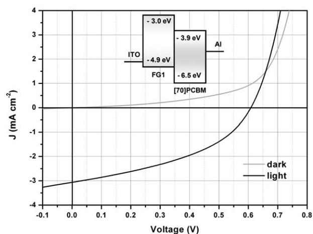
**Fig. 6** Current density voltage ( $J$ - $V$ ) characteristics and energy diagram of a **FG1**:[70]PCBM blend. The grey line was measured in the dark, the dark line under illumination (AM 1.5,  $100 \text{ mW cm}^{-2}$ ).
