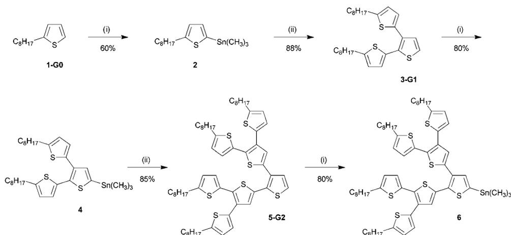
**Scheme 1** Synthesis of oligothiophene dendrons **3-G1** and **5-G2**, and stannylated derivatives **2**, **4** and **6**. *Reagents and conditions:* (i) (a) *n*-BuLi, THF,  $-78\text{ }^{\circ}\text{C}$  to  $-40\text{ }^{\circ}\text{C}$ , (b)  $(\text{CH}_3)_3\text{SnCl}$ , THF,  $-78\text{ }^{\circ}\text{C}$  to room temperature; (ii) 2,3-dibromothiophene,  $\text{Pd}(\text{PPh}_3)_4$ , DMF,  $100\text{ }^{\circ}\text{C}$ .
