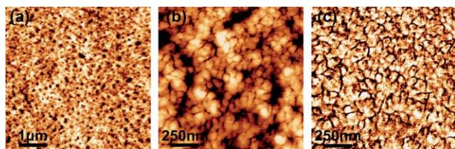
**Fig. 7** AM-AFM images (ambient conditions,  $512 \times 512$  pixels) of FG1-[70]PCBM film with a weight ratio of 1 : 2.5, as cast (a) topography,  $5 \mu\text{m} \times 5 \mu\text{m}$ . (b) topography and (c) phase,  $1.25 \mu\text{m} \times 1.25 \mu\text{m}$ .
