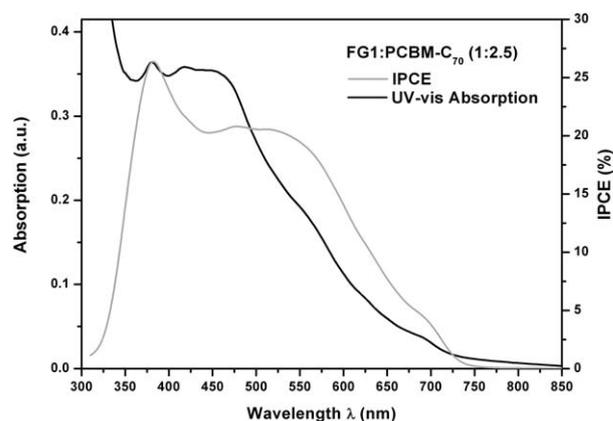
**Fig. 9** Absorption spectrum of the FG1:[70]PCBM active layer (black line) and IPCE curve of the corresponding photovoltaic cell (grey line).
