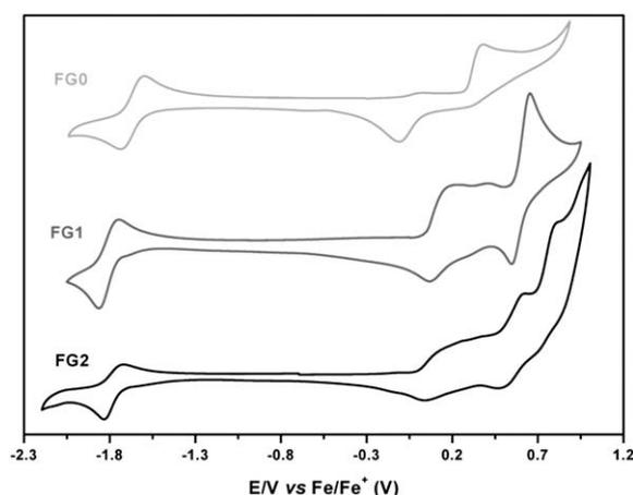
**Fig. 2** Cyclic voltammograms showing the first scans of cathodic and anodic polarization of **FG0**, **FG1**, and **FG2** at a scan rate of 20 mV s<sup>-1</sup>.
