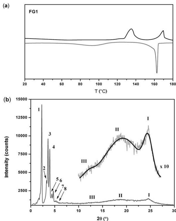
**Fig. 4** a) DSC thermogram obtained during the first heating and cooling cycles at a scan rate of  $5\text{ }^{\circ}\text{C min}^{-1}$  for **FG1**, and (b) X-ray diffractograms of **FG1** in its  $\text{Sm}_{\text{obl}}$  phase at  $150\text{ }^{\circ}\text{C}$ .
