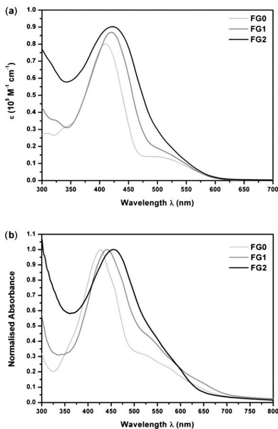
**Fig. 1** a) UV-Vis spectra of **FG0**, **FG1**, and **FG2** in chloroform solution. (b) Normalized solid-state UV-Vis spectra of **FG0**, **FG1** and **FG2** thin films cast from chlorobenzene solution.
