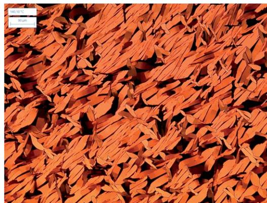
**Fig. 3** Representative polarized optical microphotograph of the texture of the mesophase shown by **FG1** at 140 °C and obtained by applying a slow cooling ( $0.5\text{ °C min}^{-1}$ ) from the isotropic phase.
