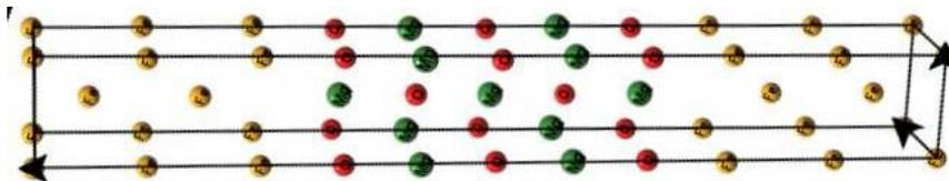
Supercell representing Fe|MgO(001) magnetic tunnel junction used in first-principles calculations
