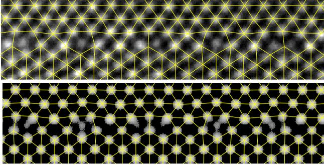
Fig. 2. – *Top*: experimental electron microscopy image superposed with atomic bonds of the model shorter than 0.32 nm. *Bottom*: simulated image calculated from the atomic positions and superposed with the same bonds (image simulation done with EMS program[11]).
