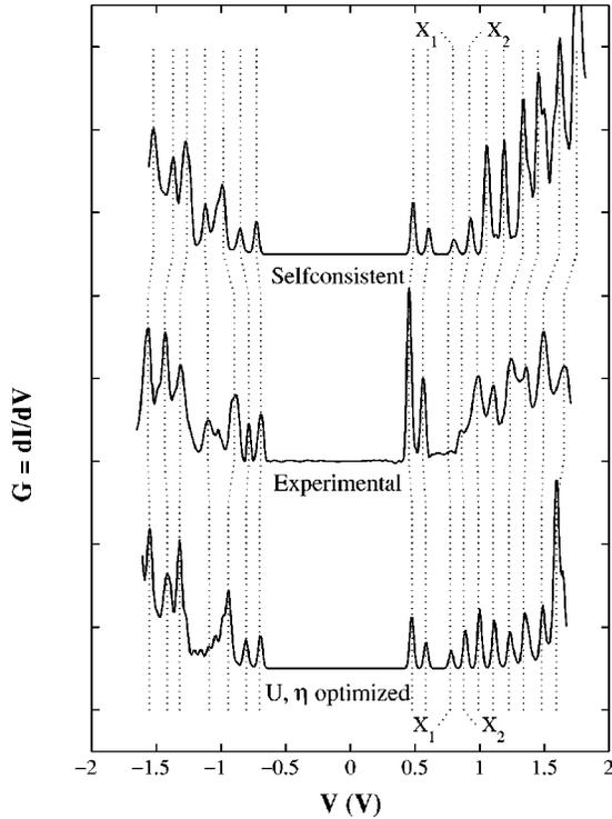
FIG. 1. Comparison between calculated and experimental differential conductance  $G(V)$  curves for a 6.4 nm diameter InAs nanocrystal. The optimized parameters for the capacitive model are  $U = 100$  meV and  $\eta = 0.9$  (see text).
