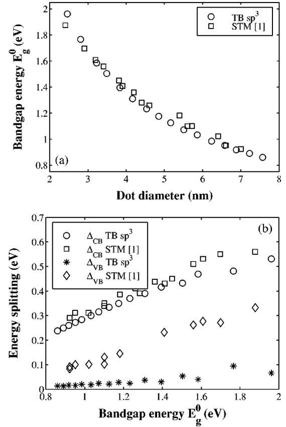
FIG. 2. (a) Comparison between the calculated (TB) and experimental [STM (Ref. 1)] band-gap energy  $E_g^0$  versus size. (b) Comparison between the calculated and experimental energy splittings  $\Delta_{CB}$  and  $\Delta_{VB}$  versus  $E_g^0$  (see text).
