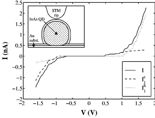
FIG. 3. Self-consistent  $I(V)$  curve for the geometry of the inset showing the electron ( $I_1^e$ ) and hole ( $I_1^h$ ) currents through junction J1.
