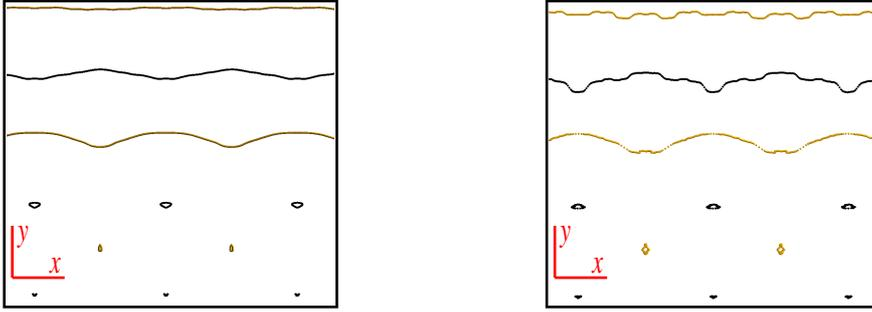
Fig. 6 – Atomic trajectories corresponding to the translation of the upper grain along  $x$  with the minimal potential energy (shown on fig. 5):  $\sqrt{2}$  gold interface without (*left*) and with  $\varepsilon = 3.5\%$  strain (*right*).
