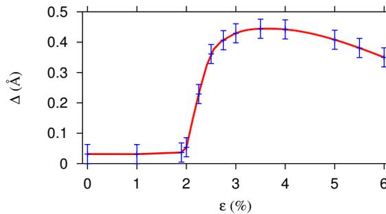
Fig. 4 – Maximum discontinuity  $\Delta$  (order parameter) of the “atomic lines”, versus the compression strain  $\varepsilon$  applied perpendicular to the interface. The “atomic lines” are calculated only at discrete points corresponding to atomic positions and the error bars correspond to the maximum separation found in the unstrained structure (approximant 239:169).
