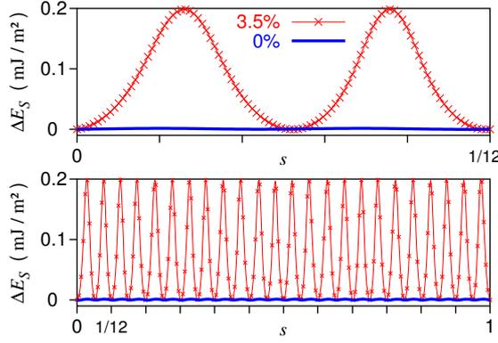
Fig. 5 – Interface energy  $\Delta E_S$  versus path coordinate  $s$  when translating one grain along the other without strain (*thick lines*) and with a 3.5 % compression strain  $\varepsilon$  applied perpendicular to the interface (*crosses*). *Bottom*: translation by one interatomic distance  $d_0 = 0.287$  nm. *Top*: translation by  $d_0/12$ . Calculation done with a “17÷12” approximant of the “ $\sqrt{2}$ ” interface.
