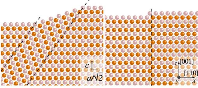
FIG. 1. (Color online) Geometry of a six atomic layer thick microtwin (left) and of an APB (right) at the top of a  $L1_0$  FePt thin film.
