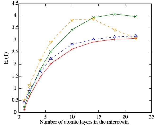
FIG. 4. (Color online) Variation of the absolute value of the depinning field as a function of the microtwin's thickness (in atomic layers), with the hypothesis that the domain wall comes from the left of the system. Results are shown for dipolar term omitted (depinning on the left:  $\Delta$  and on the right:  $\nabla$ ) and included (depinning on the left:  $+$  and on the right:  $\times$ ). The layers contain 80 atomic planes.
