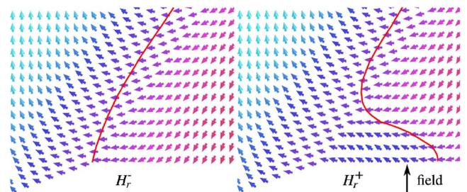
FIG. 5. (Color online) Magnetic configuration for low vertical coupling, just below the depinning field (left,  $H_r^-$ ) and at the beginning of the depinning (right,  $H_r^+$ ). It can be noticed that the magnetization is entirely in the plane of the figure (the color is a guide to the eye and the lines are the location where the magnetization is perpendicular to the field).
