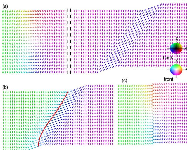
FIG. 2. (Color online) (a) Bloch wall with Néel's caps far from a microtwin. (b) Domain wall pinned in the microtwin (the line indicates the middle of the wall, where the magnetization is along  $x$ ). (c) Pinned configuration with an antiphase boundary.
