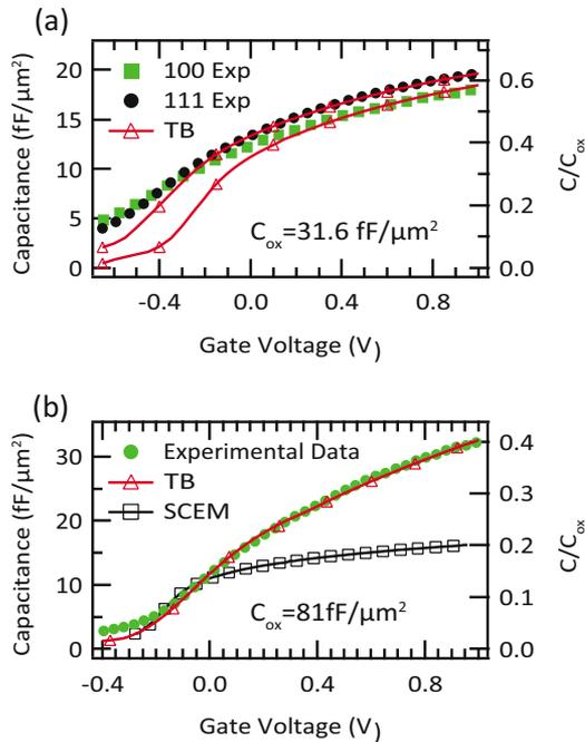
FIG. 3. (Color online) (a) Comparison between experimental and TB data for InAs (100) and (111) MOSCAPs with  $t_{\text{ox}}=6$  nm and  $C_{\text{ox}}=31.6$  fF/ $\mu\text{m}^2$ . (b) Experimental and TB/SCEM data for InAs (100) MOSCAP with  $t_{\text{ox}}=2.5$  nm,  $C_{\text{ox}}=81$  fF/ $\mu\text{m}^2$ , and  $N_d=3 \times 10^{16}$  cm $^{-3}$ .
