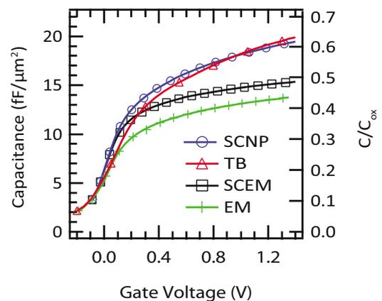
FIG. 2. (Color online) Calculated capacitance for an  $\text{In}_{0.53}\text{Ga}_{0.47}\text{As}$  capacitor with  $C_{\text{ox}}=31.6 \text{ fF}/\mu\text{m}^2$  and  $N_d=7.2 \times 10^{16} \text{ cm}^{-3}$ .
