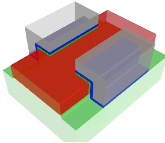
**Model for a simulated qubit** : A silicon wire (red) is controlled by two gates (gray) isolated by oxides (green/blue). An electron can be stored and manipulated under each gate. Coulomb and tunnel interactions between these electrons entangle their dynamics.
