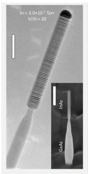
Image of an InAs-on-GaAs nanowire taken by transmission electron microscope (scale bar 100 nm). The dark droplet at the top is the gold catalyst. Inset: image of a standing nanowire from the same sample taken by scanning electron micrograph (scale bar 200 nm, 30° tilt).
