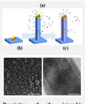
Description of the internship Growth. methodology. (a) InAs nanowires will be grown by the VLS mechanism using gold catalysts. Then a shell of V will be fabricated by switching the growth mode to 2D growth. (b) Morphology. SEM image of a sample of InAs/Al nanowires with polycrystalline Al shells. (c) Structure. TEM image of a hybrid Si/III-V core-shell nanowire.
